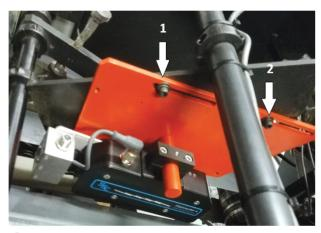
**3** Install new orange bracket with sensor, using ¼" hex wrench, install screws (1&2) removed in step 1 above. Position sensor and bracket as shown in picture above.
