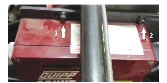
■ Using ¼" hex wrench, remove screws (1 &2), freeing laser from mount. Retain these screws for installation of new sensor.
