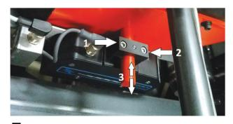
**5** ■ If necessary, adjust sensor between the belts, by loosening screws (1&2) with 5mm hex wrench, and sliding on shaft (3).
