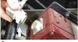
**2** Loosen collar (1) and remove connector from laser. Remove Quipp™ Laser.
