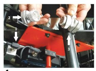
**4** Install connector (1). Screw together connectors 2 and 3.
