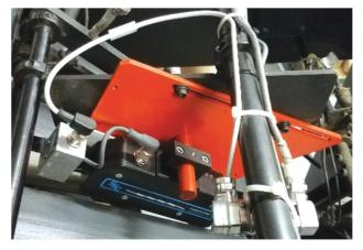
**6** ■ Secure cables away from moving parts with cable ties.
